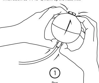
• Push the reinforced base of the cable into the head until enough of the battery tube is exposed to grasp
